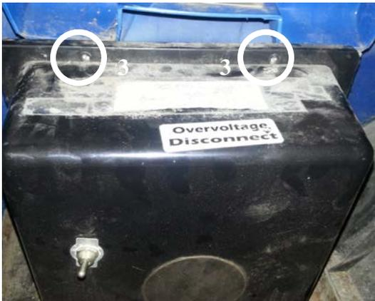
1. The control Panel Assembly is held in place by two M8 Nuts, these nuts are located underneath the cart. Remove them.
