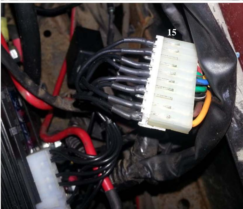
12. Reconnect the motor A1 wire to the B+ terminal of the controller and the A2 wire to the M-. (**Avoid placing wiring in the NCZ-no cable zone**)
