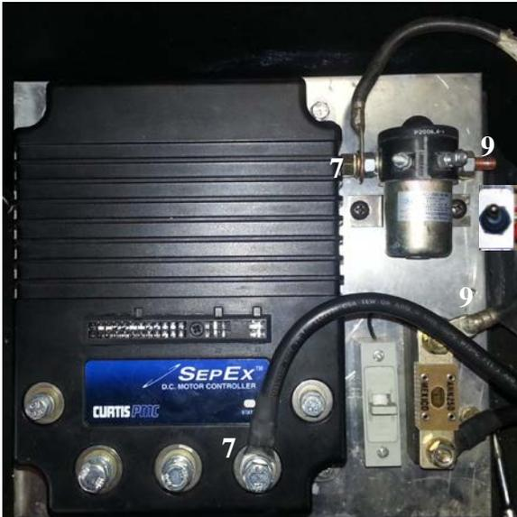
7. If using the old contactor connect the terminal closest to the controller (large diameter pole) to the B+ terminal of the control using supplied 4AWG wire.
